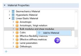
This lets you define the bulk modulus and shear modulus for the copper in your model.
