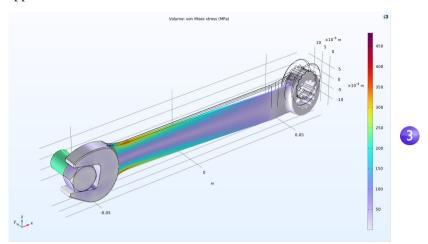
For our purposes we are not interested in the stress in the bolt. We can selectively visualize the stress in just the wrench by adding a **Selection** node.
