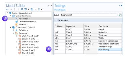
5 Select File > Save As and save the model with a new name, busbar box I.mph.
