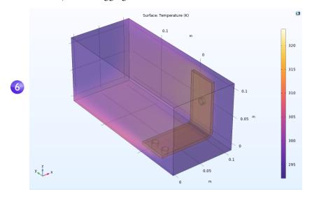
The **Temperature Surface** plot that displays in the **Graphics** window shows the temperature in the busbar and in the surrounding box. You can also see that the temperature field is not smooth due to the relatively coarse mesh. A good strategy to get a smoother solution would be to refine the mesh to estimate the accuracy.
