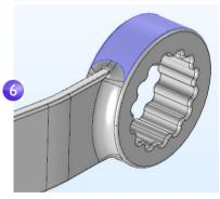
7 In the Settings window for Boundary Load, under Force, select Total force as the Load type and enter -F in the text field for the z component. The negative sign indicates the negative z direction (downward). With these settings, the load of 150 N will be distributed uniformly across the selected surface.
