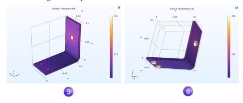
The temperature distribution is laterally symmetric with a vertical mirror plane running between the two lower titanium bolts and cutting through the center of the upper bolt. In this case, the model does not require much computing power and you can model the entire geometry. For more complex models, you can consider using symmetries to reduce the computational requirements.
