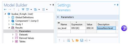
3 For the Isothermal Contours (ht) I plot group, in the Settings window for the Isosurface plot, change the Entry method to Levels. For the Levels expression field, type iso level.
