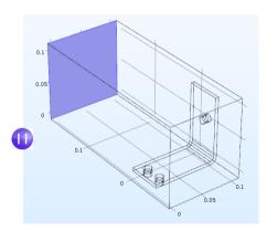
The settings for the busbar, the bolts, and the **Electric Potential I** and **Ground I** boundaries have retained the correct selection, even though you added the box geometry for the air domain. To confirm this, in the model tree under **Electric Currents**, click the **Electric Potential I** and the **Ground I** nodes to verify that they have the correct boundary selection.
