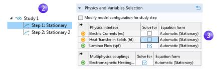
3 In the Settings window for Stationary, locate the Physics and Variables Selection section. In both the Electric Currents (ec) and the Heat Transfer in Solids (ht) rows, click to change the check mark ☐ to an ☐ in the Solve for column, removing the Joule heating effect from Step 1.
