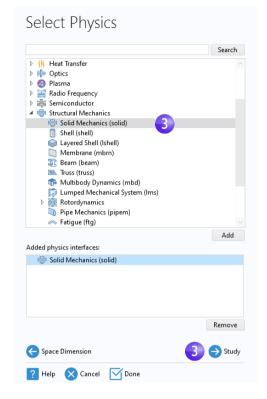
**General Studies** and other preset studies have solver and equation settings adapted to the selected physics, which is, in this example, **Solid Mechanics**. A **Stationary** study is used in this case — there are no time-varying loads or material properties.
