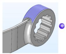
5 In the Settings window for Boundary Load, under Force, select Total force as the Load type and enter -F in the text field for the z component.
