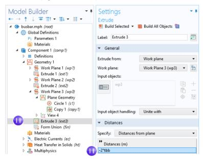
The geometry and geometry sequence should match the figures below. Click the **Save** button  $\square$  and name the model busbar.mph.
