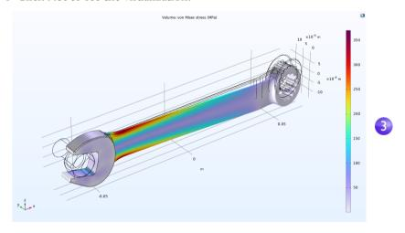
For a typical steel used for tools like a wrench, the yield stress is about 600 MPa, which means that we are getting somewhat close to plastic deformation for our 150 N load (which corresponds to about 34 pounds force). You may also be interested in a safety margin of, say, a factor of three. To quickly assess which parts of the wrench are at risk of plastic deformation, you can plot an inequality expression such as solid.mises>200[MPa].
