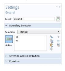
Next, continue with the flow settings. You need to indicate that fluid flow only takes place in the fluid domain and then set the inlet, outlet, and symmetry conditions. Do this by first removing all domains from the selection and then adding the air domain.
