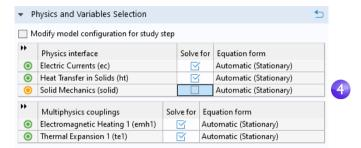
Now, repeat these steps to remove **Electric Currents (ec)** and **Heat Transfer in Solids (ht)** from the second study step.
