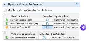
5 Right-click the **Study I** node ∞ and select **Compute** = (or press F8 or click **Compute** in the ribbon). This will now automatically create a new solver sequence that solves for laminar flow and then Joule heating.
