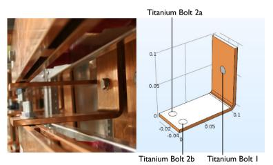
The goal of your simulation is to precisely calculate how much the busbar heats up. Once you have captured the basic multiphysics phenomena, you will have the chance to investigate thermal expansion that generates structural stresses and strains in the busbar and the effects of cooling by an air stream.
