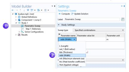
The Sweep type is used to control parametric sweeps with multiple parameters. You select between sweeping for All combinations of the given parameters, a subset of Specified combinations, or Parameter switch. The option Parameter switch makes it possible to sweep over Cases for Parameters as defined in Global Definitions, as shown below.
