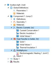
heating effect is set in the **Electromagnetic Heating** node under the **Multiphysics** node. The **Initial Values** node, found in both the **Electric Currents** and **Heat Transfer in Solids** interfaces, contains initial guesses for the nonlinear solver for stationary problems and initial conditions for time-dependent problems.
