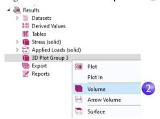
3 In the Settings window for Volume, click the Replace Expression button and select Model > Component I > Solid Mechanics > Stress > solid.mises-von Mises stress - N/m² by double-clicking. When you know the variable name beforehand, you can also directly enter solid.mises in the Expression field. Now edit this expression to:
