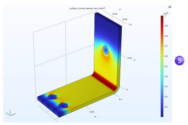
**6** Click and drag the busbar in the **Graphics** window to view the back. Continue rotating the image to see the high current density around the contact surfaces of each of the bolts.
