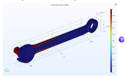
You may have noticed that the manufacturer, for various reasons, has chosen an asymmetric design for the wrench. Because of that, the stress field may be different if the wrench is flipped around. Try now, on your own, to apply the same force in the other direction and visualize the maximum von Mises stress to see if there is any difference.
