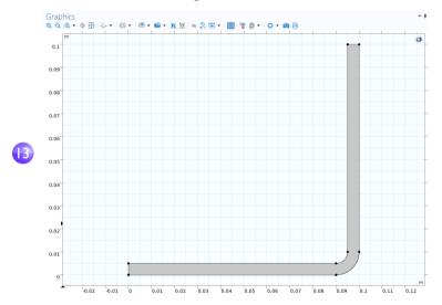
In the Design Module you will find tools for interactive drawing and dimensioning of fillets and general 2D sketches.
