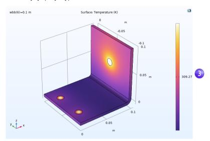
The plot may look a bit different depending on which version you are running. Compare the wider busbar plot to the temperature for wbb=0.05[m] (5[cm]). For this purpose, you can reuse one of the previously defined plot groups.
