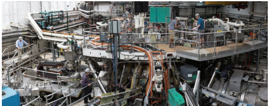
Figure 2. The DIII-D tokamak is surrounded by complex systems and components, which are exposed to strong magnetic fields.
