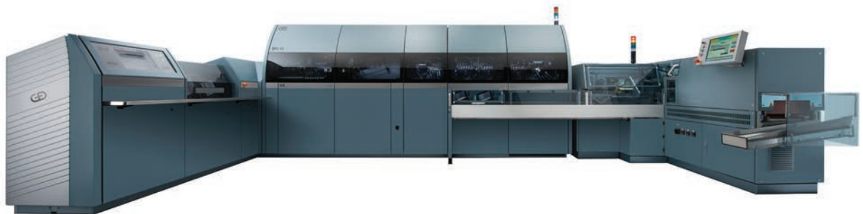
Figure 1. The BPS X9, the fastest banknote processing system in the world, has a processing speed of 44 banknotes per second and can achieve an effective throughput of more than 150,000 banknotes per hour. The dimensions of the central module are 1.9 m x 5.7 m (H x W).
