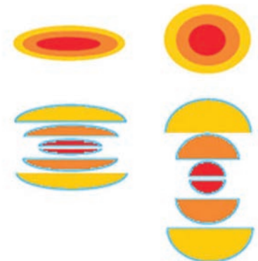
Figure 6. Simplified finite multilayer representation of the GRIN with decomposition in equivalent lens. Far vision is pictured on the left, near vision on the right. Colors represent the value of the refractive index with the highest values in red.
