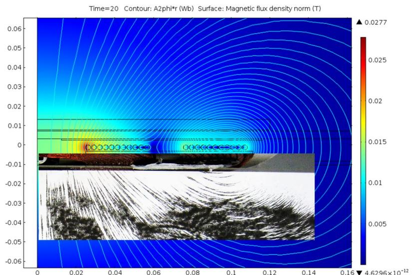
Comparison between results from COMSOL Multiphysics® software (magnetic flux density norm) and experimental field lines can be used to test other coil designs before building a prototype.
