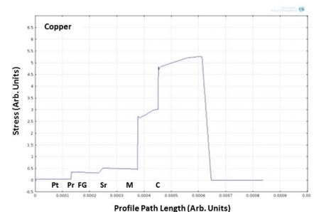
Relative stress in arbitrary units was plotted through the depth of the composite structure layups containing either aluminum (left) or copper EMF (right).
