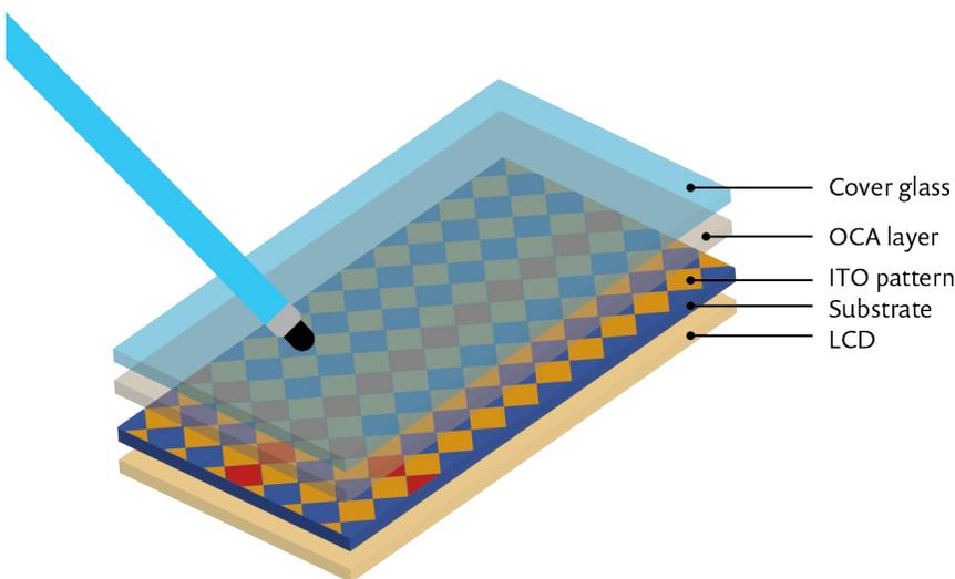
Typical touchscreen sensor stack-up, which contains an LCD layer followed by a substrate, a pattern of horizontally and vertically aligned diamond-shaped ITO electrodes, and finally an optically clear adhesive layer that bonds the glass cover onto the screen.
