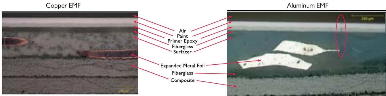
Photo micrographs of the composite structure layups after exposure to moisture and thermal cycling. At left, the results for the copper EMF and at right, the aluminum.
