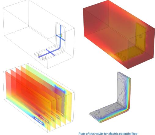
Plots of the results for electric potential (top left), temperature (top right), velocity (bottom left), and pressure (bottom right)
