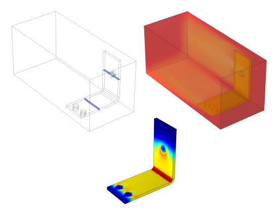
Plots of the results for electric potential (left), temperature (top right), and current density (bottom right).
