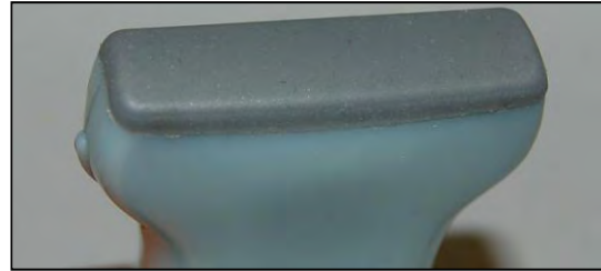
Figure 4: Complete probe head, with silicon lens and covers.
