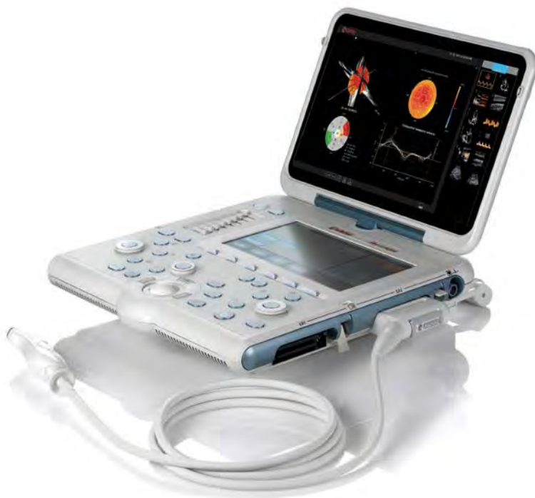
Figure 1. The performance of ultrasonic diagnostic systems such as MyLabOne (left) depends heavily on probes placed on the skin (right).
