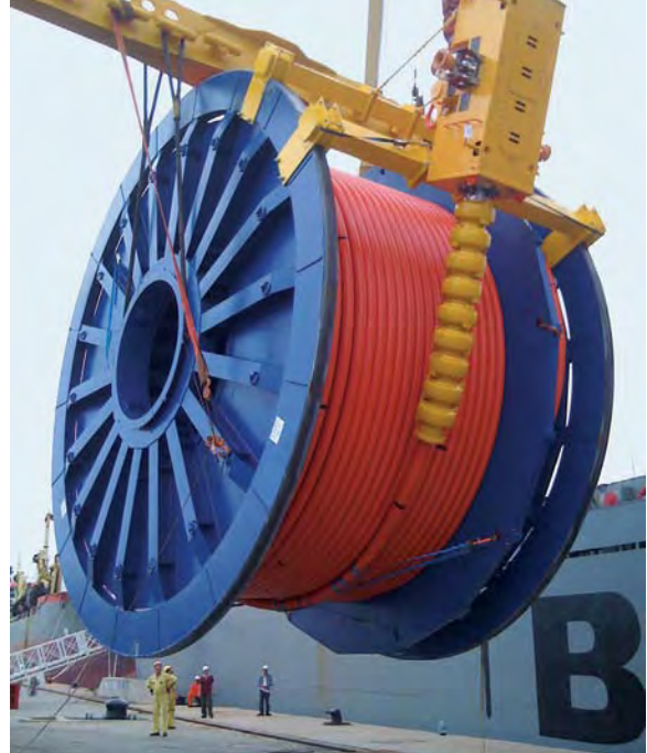
An umbilical cable on a drum ready to be placed on a ship for laying.
